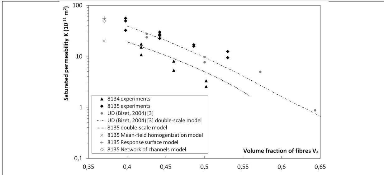
**Figure 1:** Comparison of the different methods for determination of longitudinal warp permeability in saturated regime.
